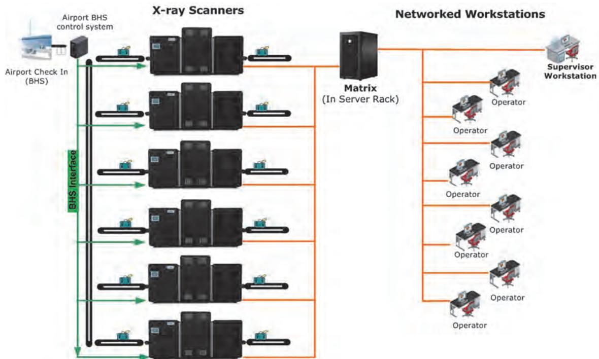
Figure 2 BHS Integrated - Multiple RTT110's Scanner with Multiple Networked Workstations
