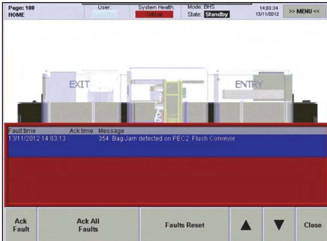
Figure 15 Bag Jam Fault - Acknowledging Fault
