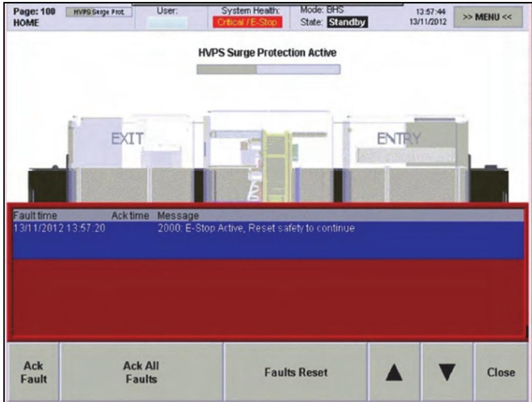
Figure 19 Fault pop up window - displays E-stop Fault details
