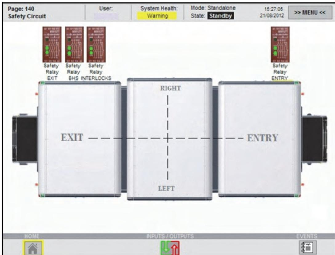
Figure 20 HMI Machine Control toolbar, Safety Circuit page
