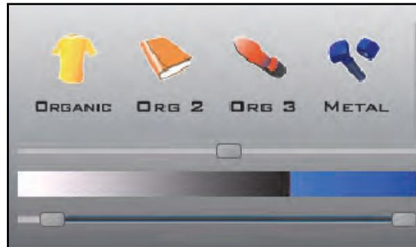
A graph display that allows the user to observe how density values are distributed in the image. (Density determines the color and transparency of each image pixel.)
