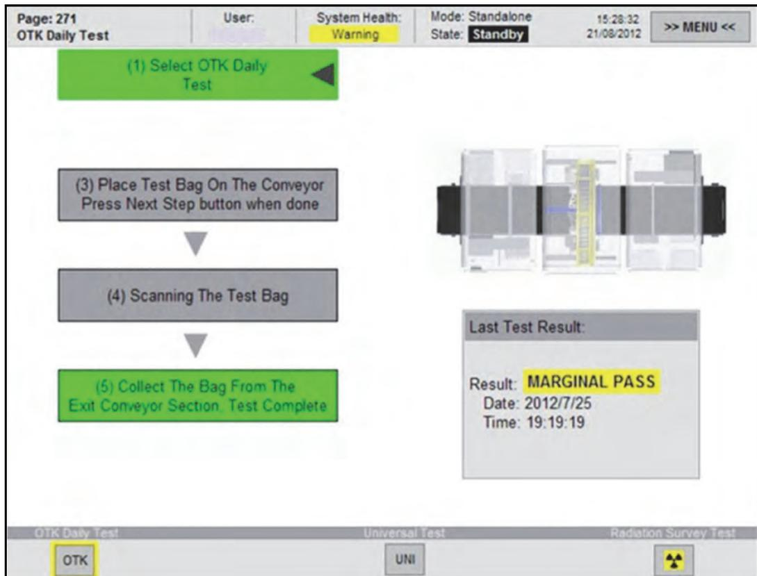
Figure 20 HMI Menu, Service option, Tests - OTK Daily Test
