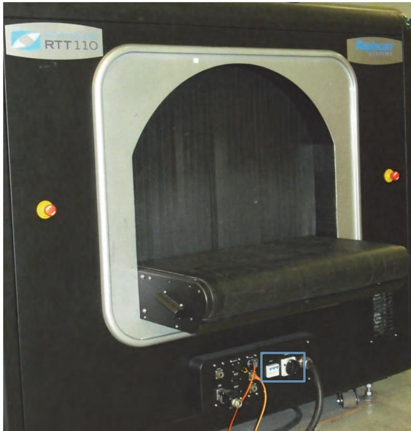
*Figure 1 RTT110 - Main Circuit Breaker (MCB) and Mains Isolator switch location*
