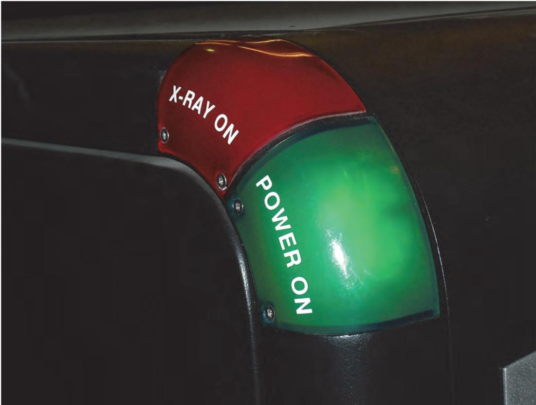
*Figure 2 RTT110 Safety lamps, Power On lamp illuminated*
