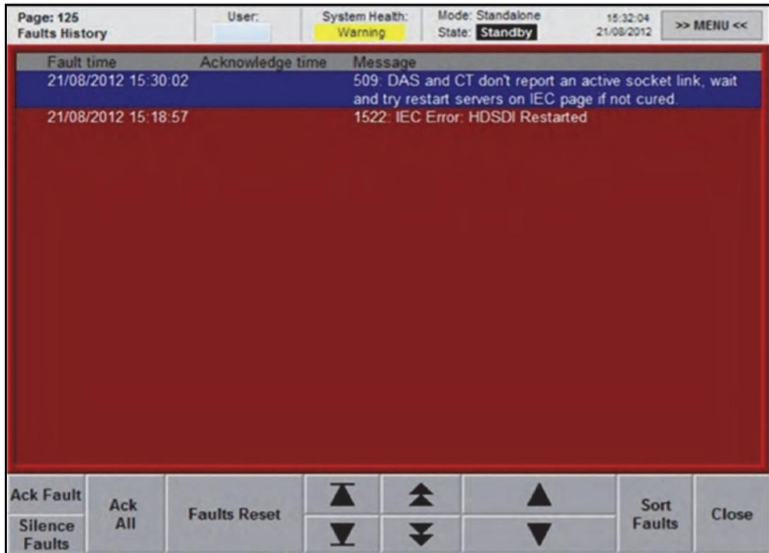
Figure 12 HMI, Machine Control toolbar, Faults History page
