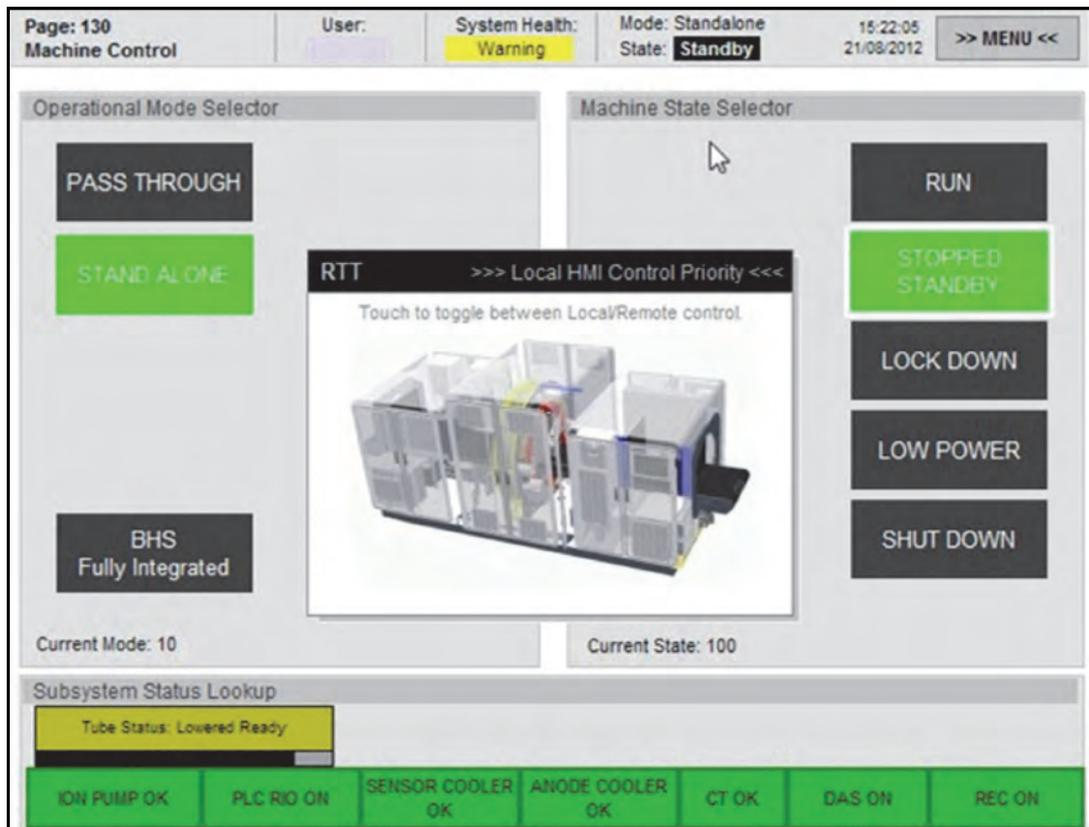
Figure 7 HMI, Machine Control toolbar, Machine Control page
