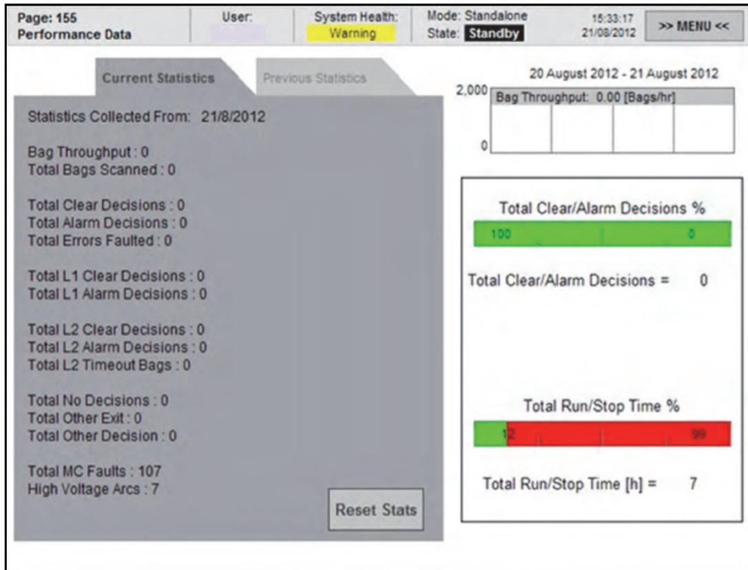
Figure 15 HMI, Machine Control toolbar, Performance Data page
