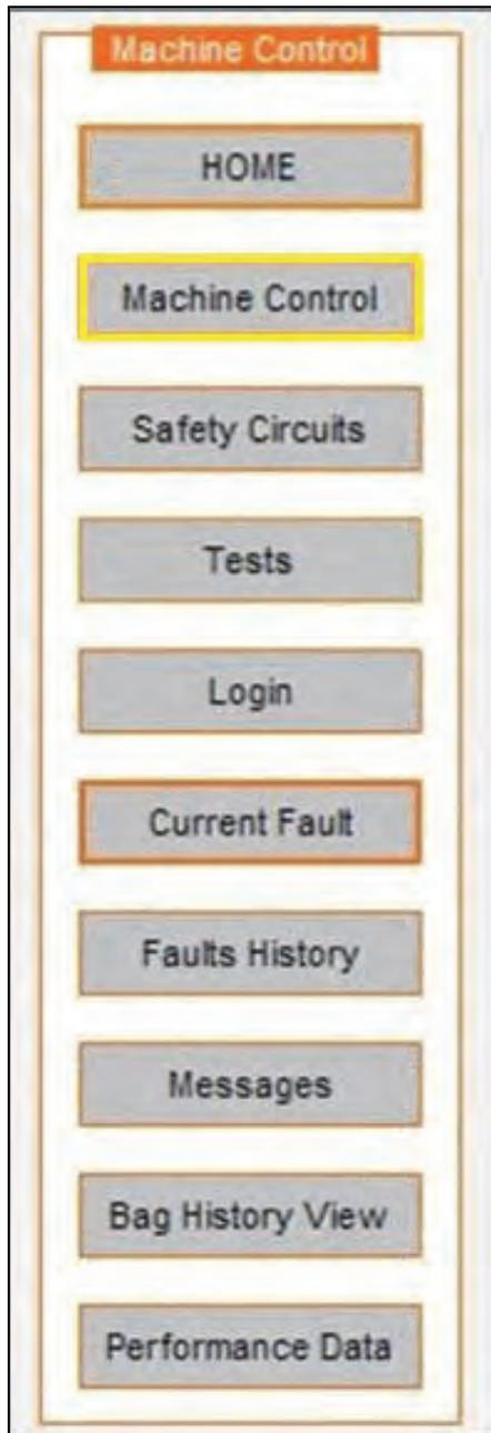
Figure 6 HMI Page Navigation Menu, Machine Control toolbar
