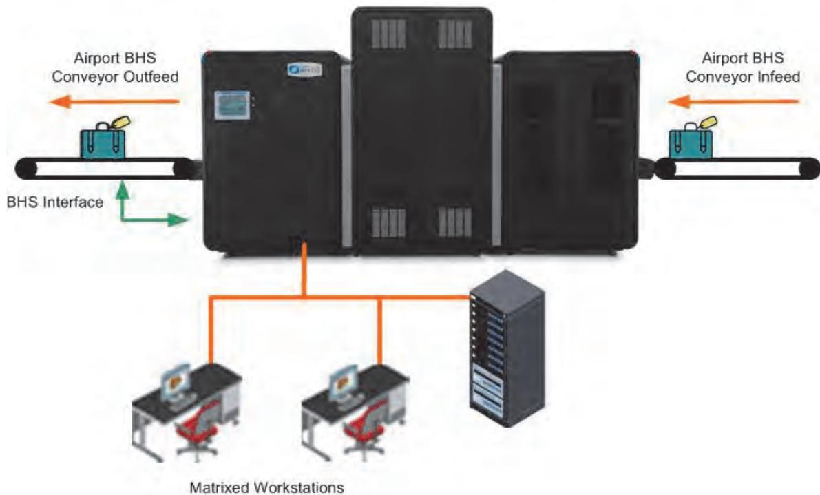
*Figure 3 Single RTT110 - Integrated with Multiple Matrixed Workstations*
