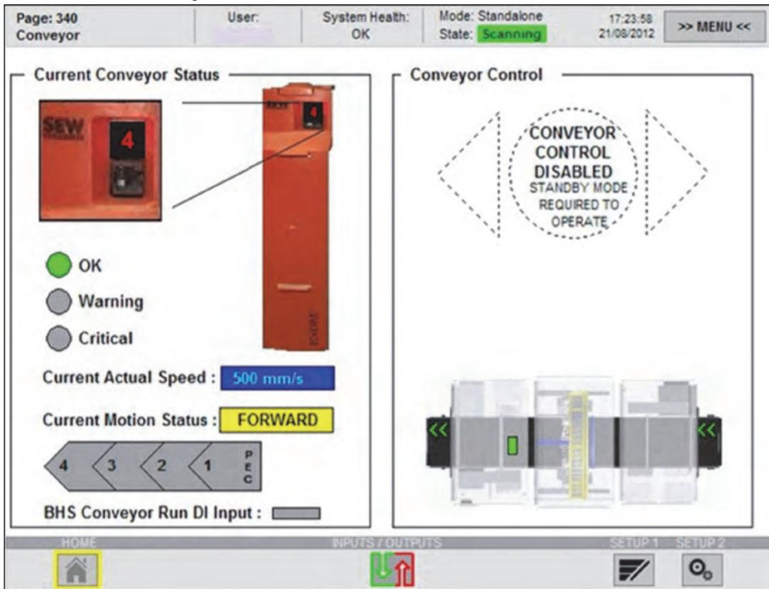
Figure 16 HMI, Subsystems toolbar, Conveyor page
