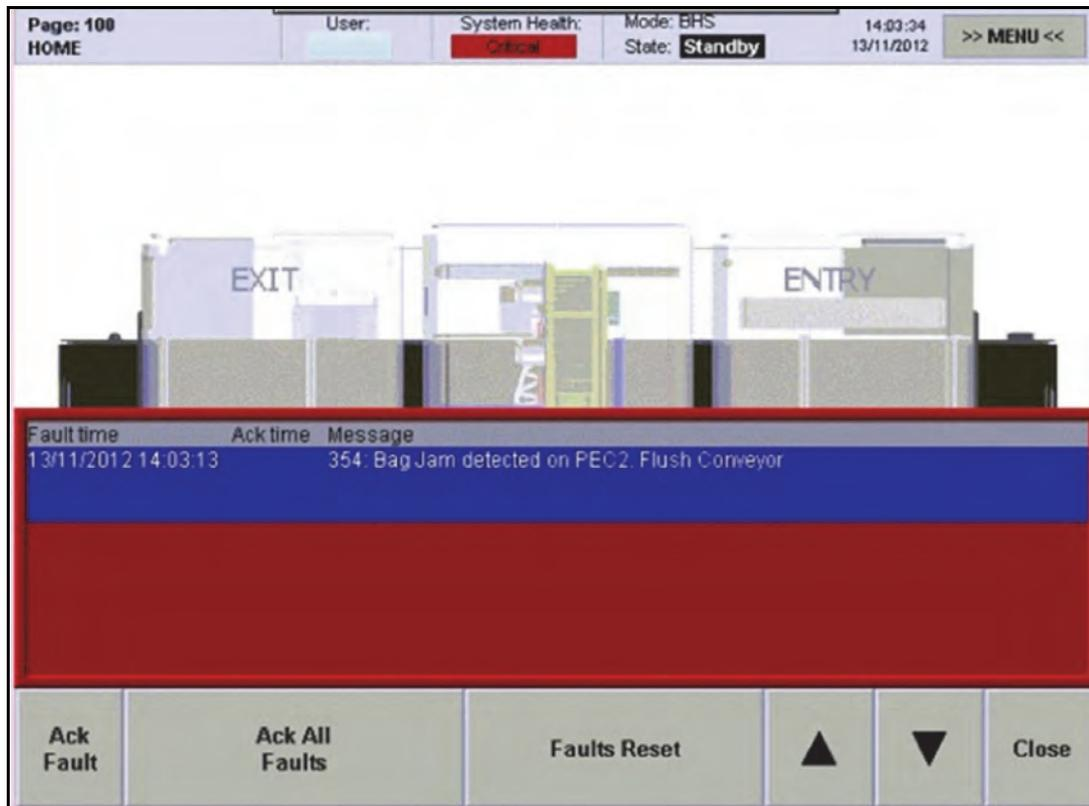
Figure 18 HMI Fault - Bag Jam Active
