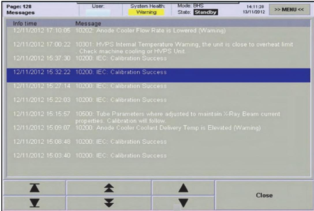
Figure 13 HMI, Machine Control toolbar, Messages page
