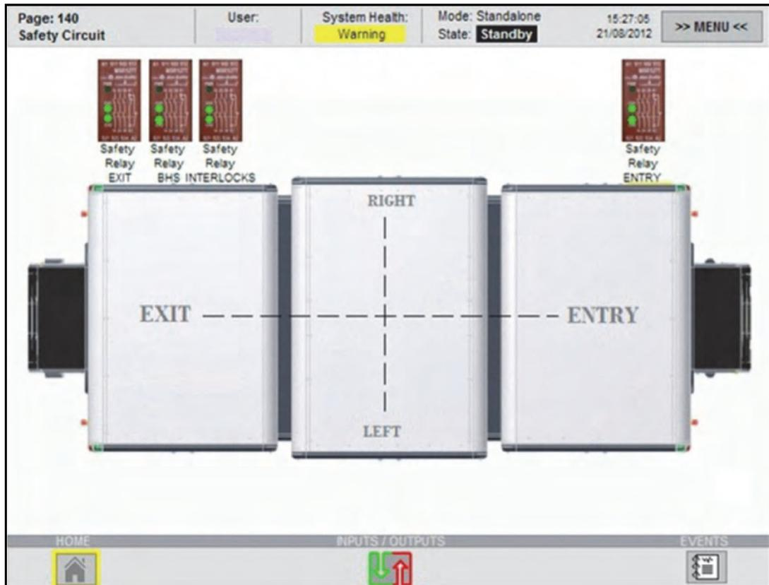
Figure 8 HMI, Machine Control toolbar, Safety Circuit page
