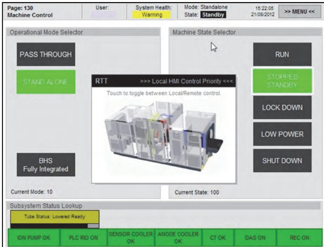
Figure 6 HMI, Machine Control toolbar, Machine Control page
