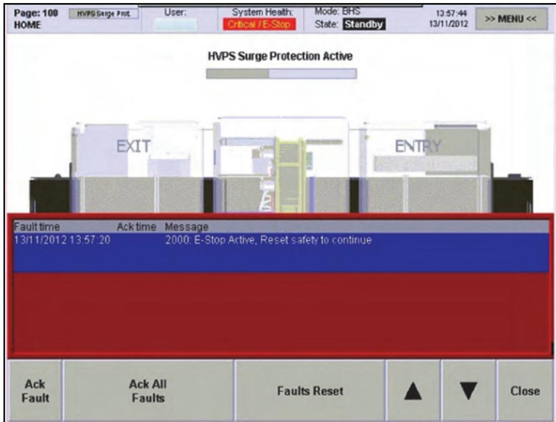
Figure 16 HMI Fault - E-stop Active
