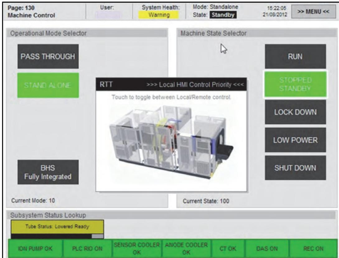
Figure 7 HMI, Machine Control toolbar, Machine Control page
