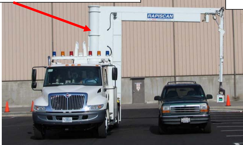
Figure 5-3: Adjustable Boom Height Options Showing Truck Height Option
