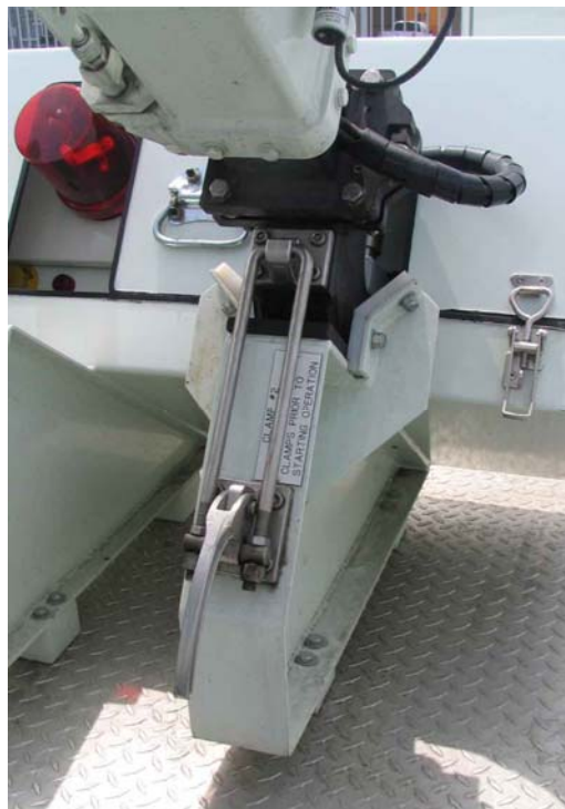
Figure 12-6: Clamp #2 beneath the Source Enclosure Box
