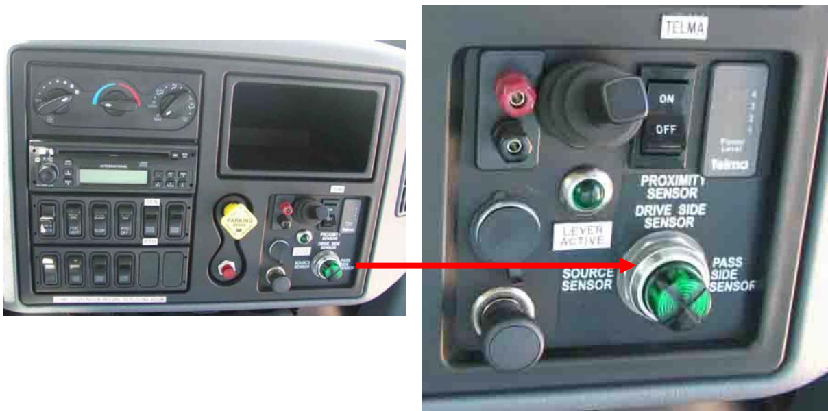
Figure 5-14: Proximity Sensor Light on Dashboard
