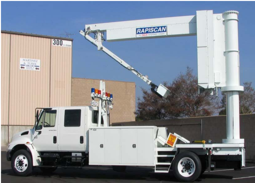
Figure 7-11: Deploying the Boom Sequence Step 3
