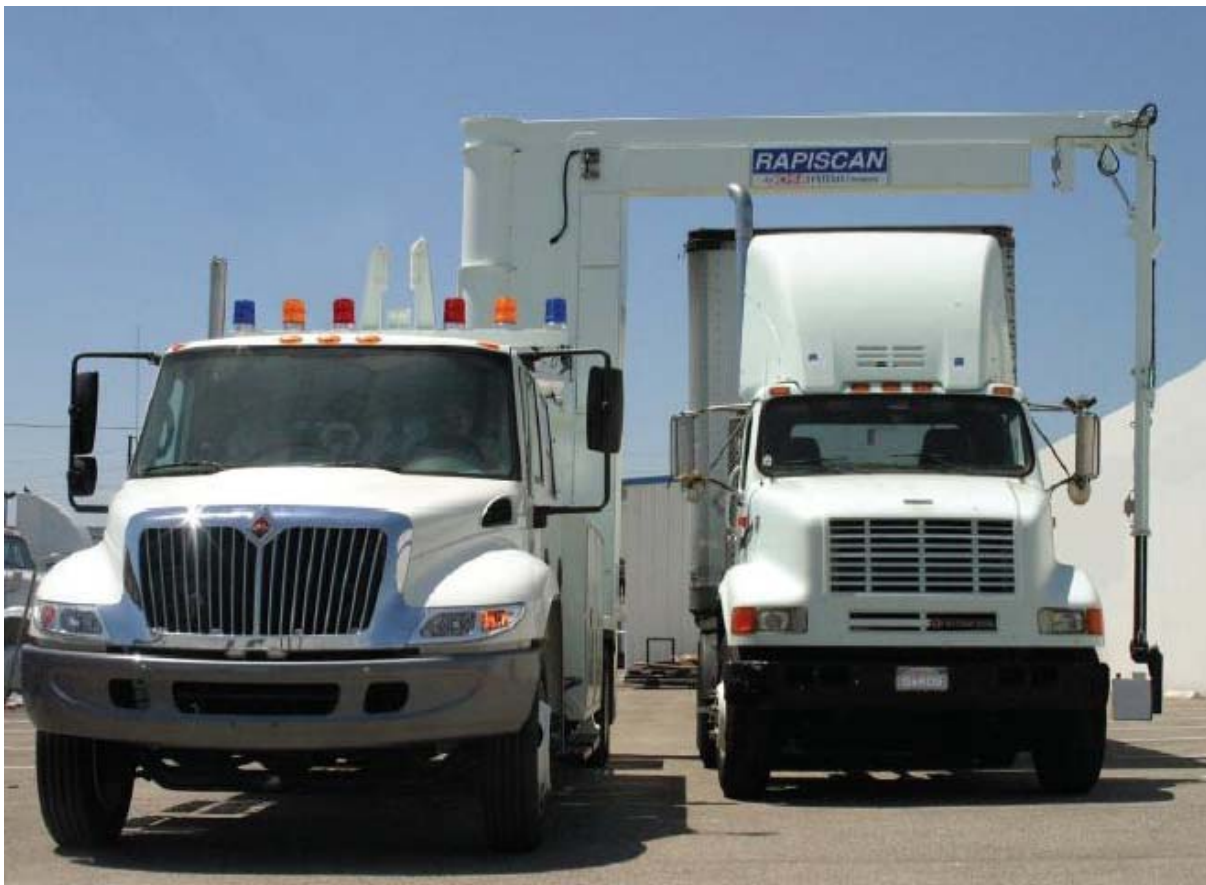
Figure 1-1: GaRDS Mobile Truck – Operational Configuration
