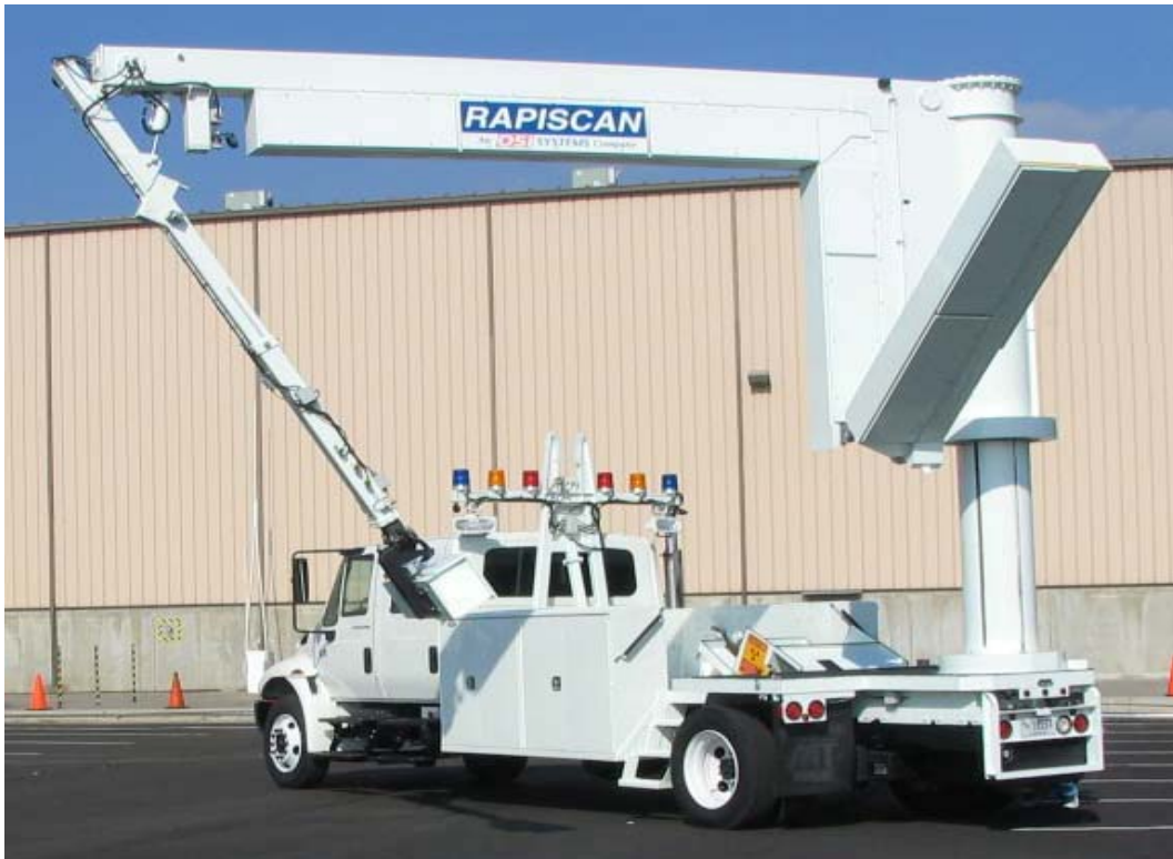
Figure 7-13: Deploying the Boom Sequence Step 5
