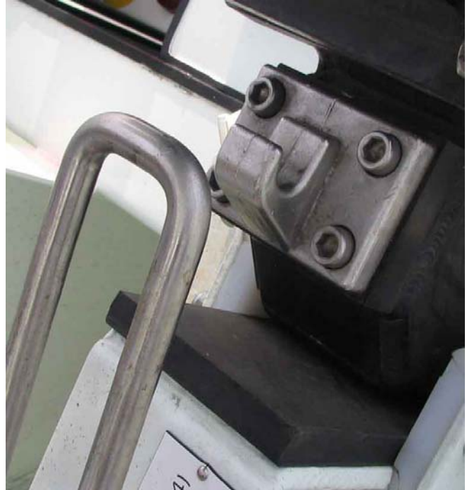
Figure 12-8: A clamp NOT properly locked
