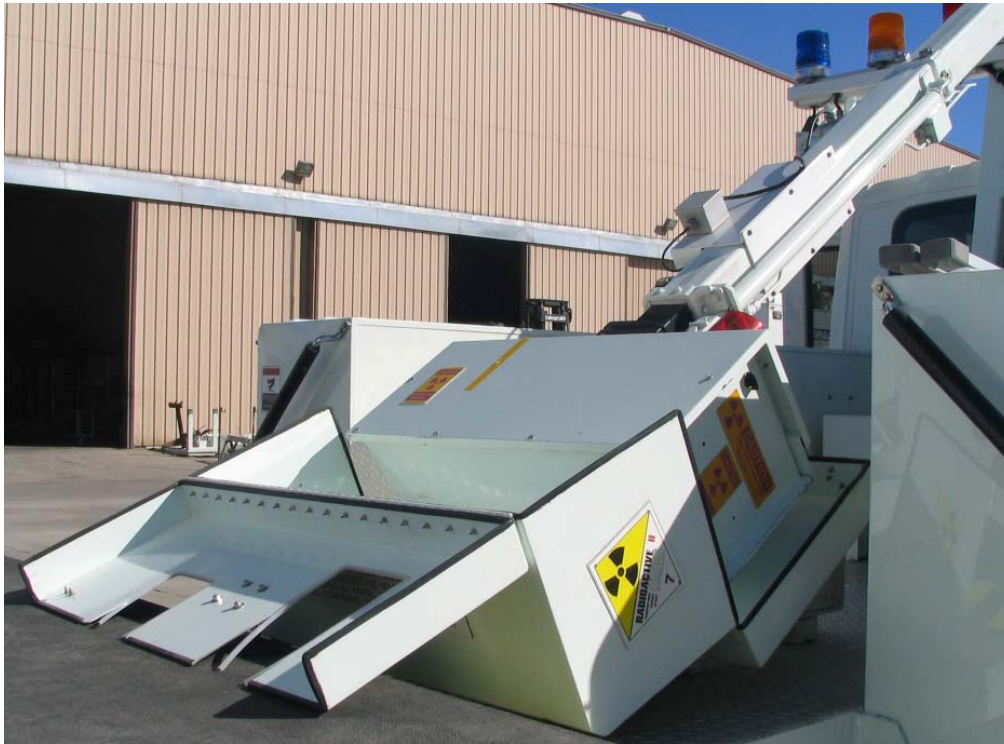
Figure 12-3: Source Transportation Box
