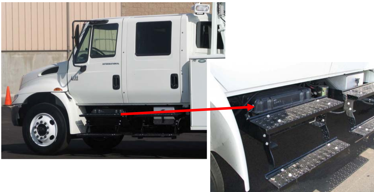
Figure 5-23: Dual Truck Batteries
