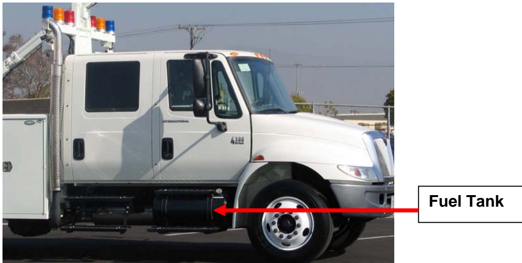
Figure 5-22: Diesel Fuel Tank
