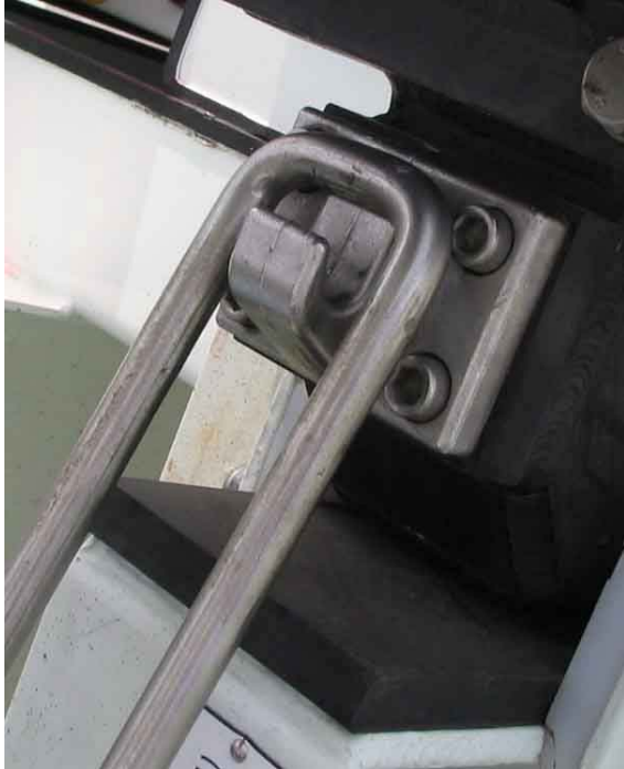
Figure 12-8: A clamp NOT properly locked
