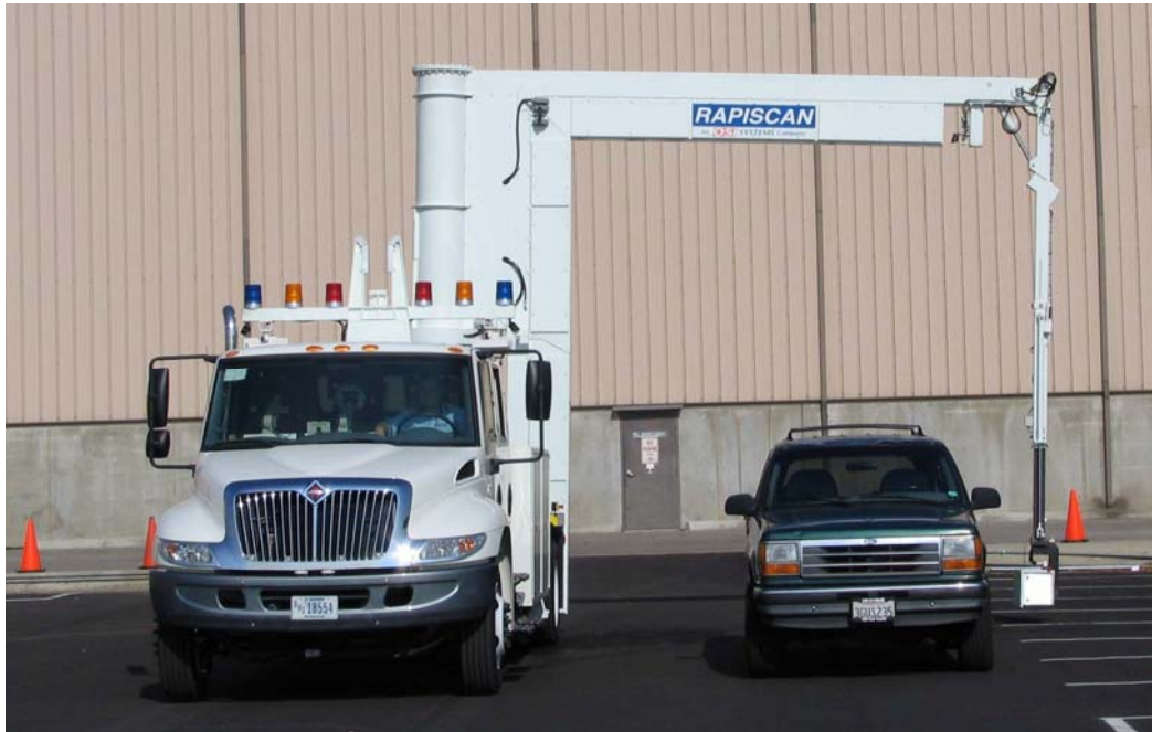
Figure 9-1: GaRDS Mobile Truck Performing Scanning Operations
