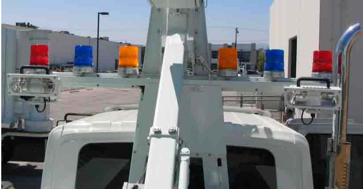
Figure 12-10: Light bar showing the Blue Strobe Lights
