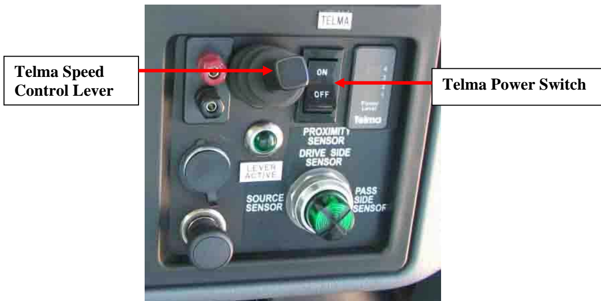
Figure 5-12: Telma Power Switch and Speed Control Lever
