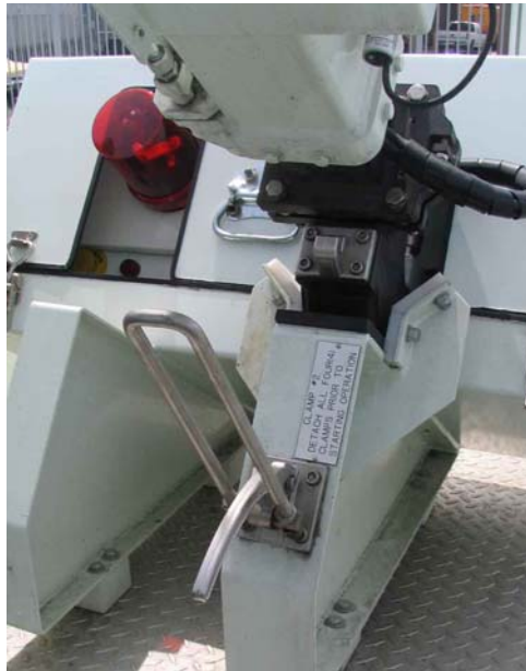
Figure 7-3: Clamp #2 beneath the Source Enclosure Box
