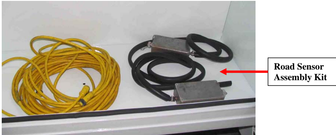
Figure 10-2: Road Sensor Assembly Kit in the Rear Storage Cabinet
