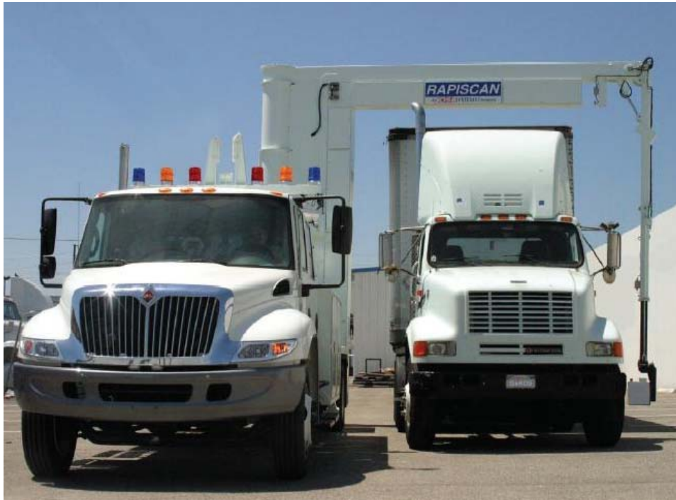
Figure 8-1: GaRDS Mobile Truck during Operations –Operational Configuration
