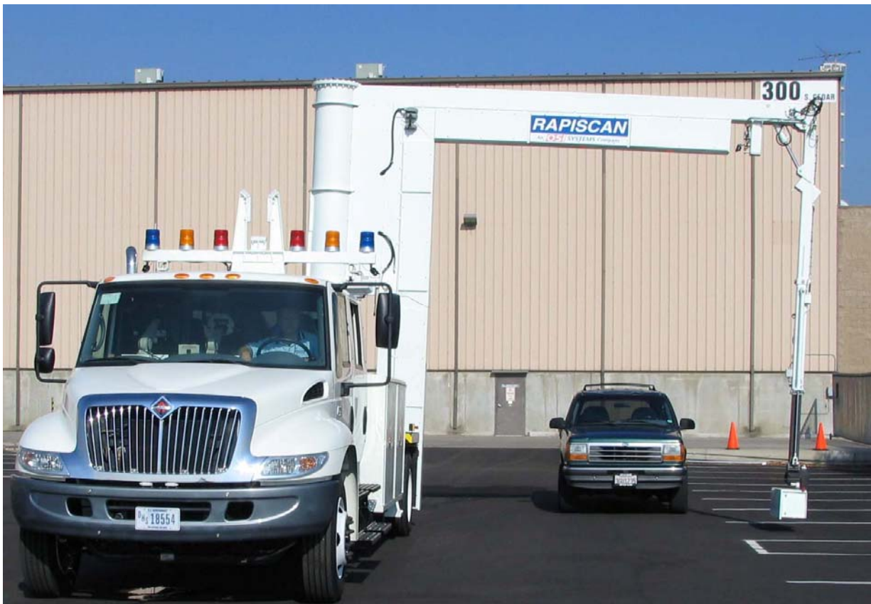
Figure 9-4: GaRDS Mobile Truck Finishing Scanning Operations
