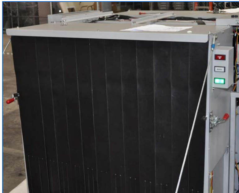
Figure 23: Curtains and Light Indicator Box
