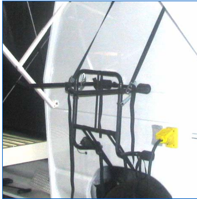
Figure 53: Support Rack Installed
