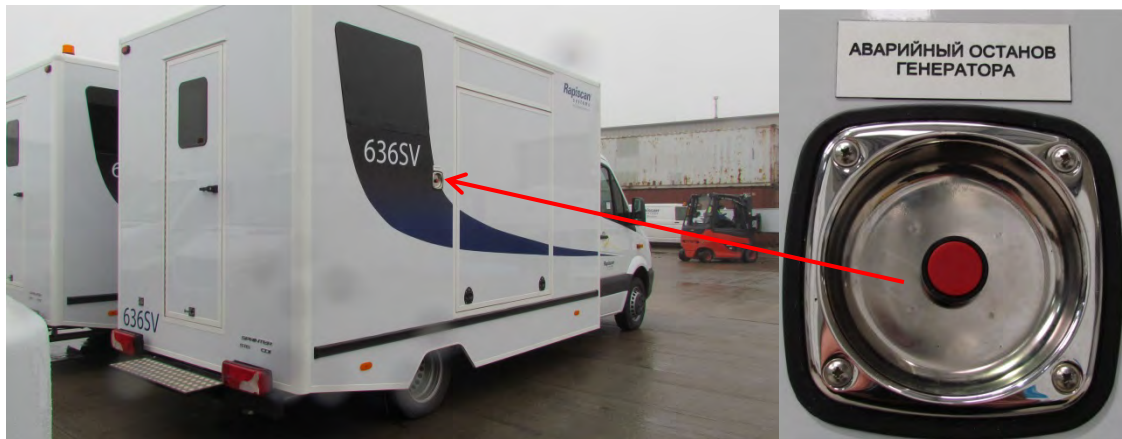
Figure 6-3 Van Mounted Emergency Stop
