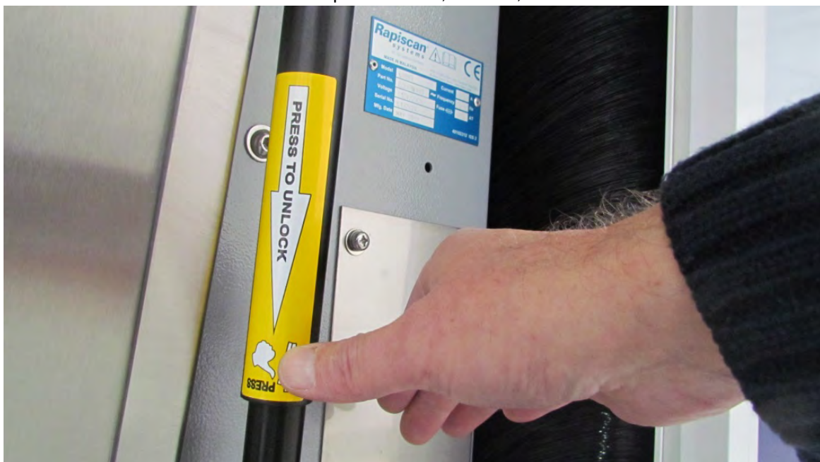
Figure 7-4 Pushing the Suspension Strut Sleeve
