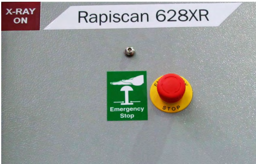
Figure 4-13 Emergency Stop (Typical)
