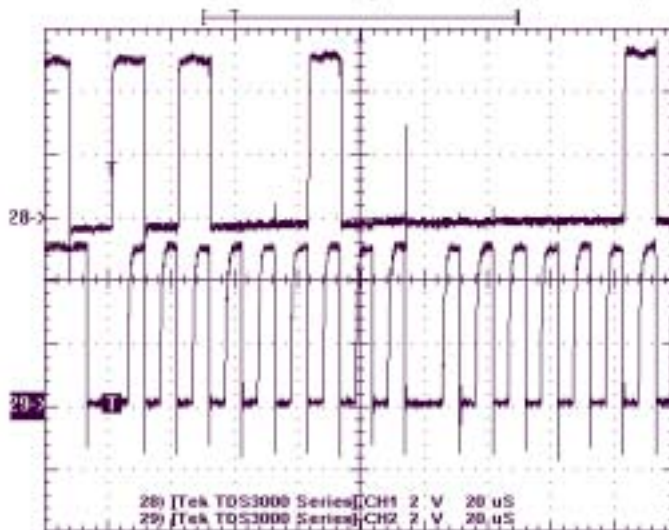
MDPU 5007: I2C clock and data during menu scroll (IC5 pins 6 and 5)
