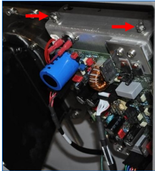
Figure 267: Controller Mounting Bolts
