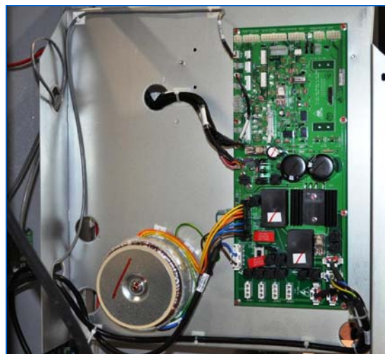
Figure 252: PDI Board on Inside Panel of Electronics Chassis
