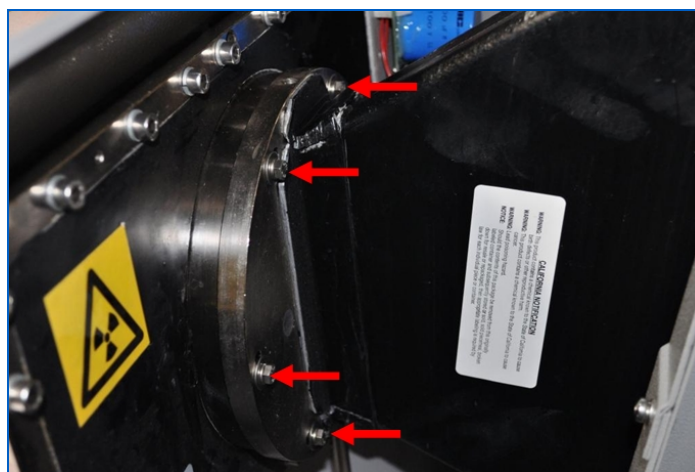
Figure 268: Collimator Mounting Bolts
