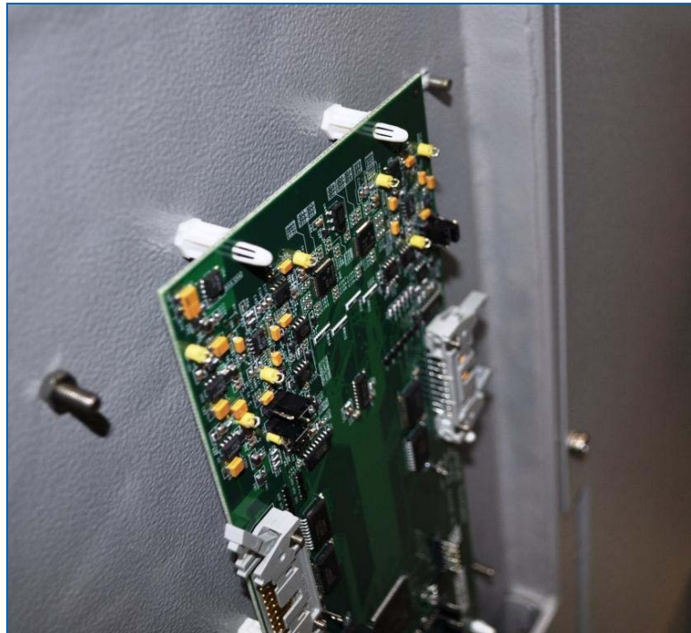
Figure 316: ADC Board Standoffs
