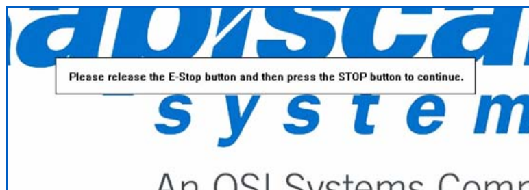
Figure 117: E-Stop Release Message
