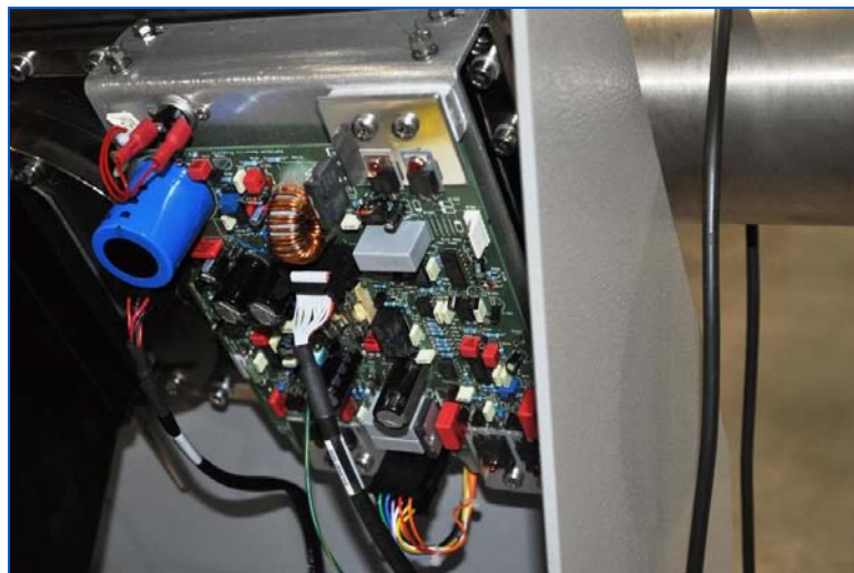
Figure 286: 180 kV Generator X-ray Control PCB (P/N: 91001)
