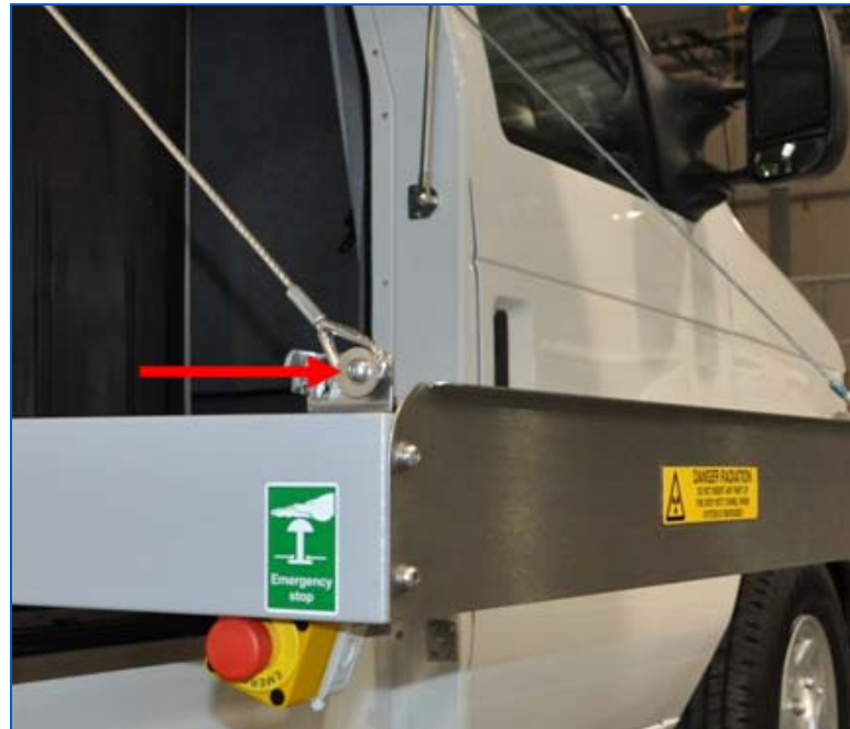
Figure 337: Conveyor Cable Bolt
