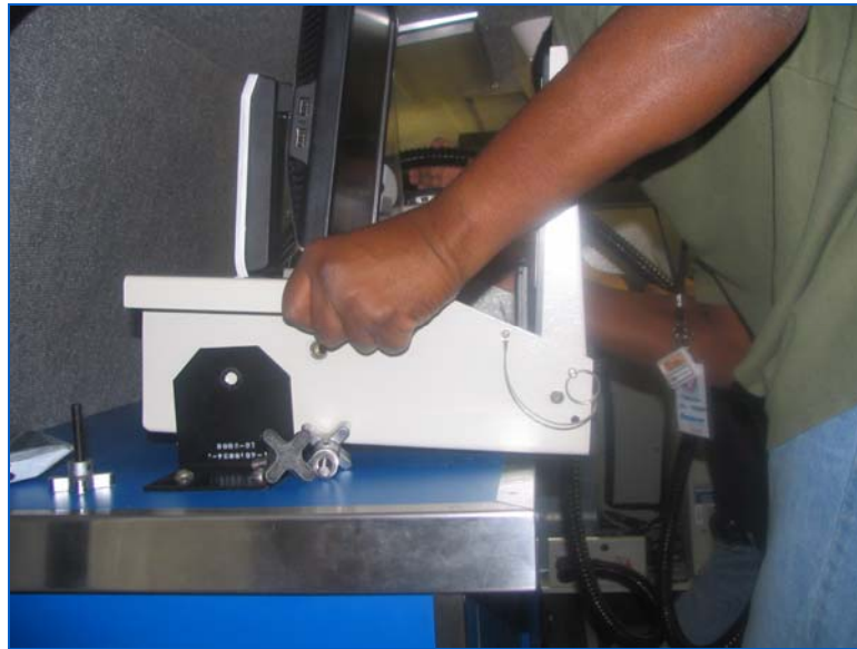
Figure 63: Lifting Monitor/Keyboard Assembly
