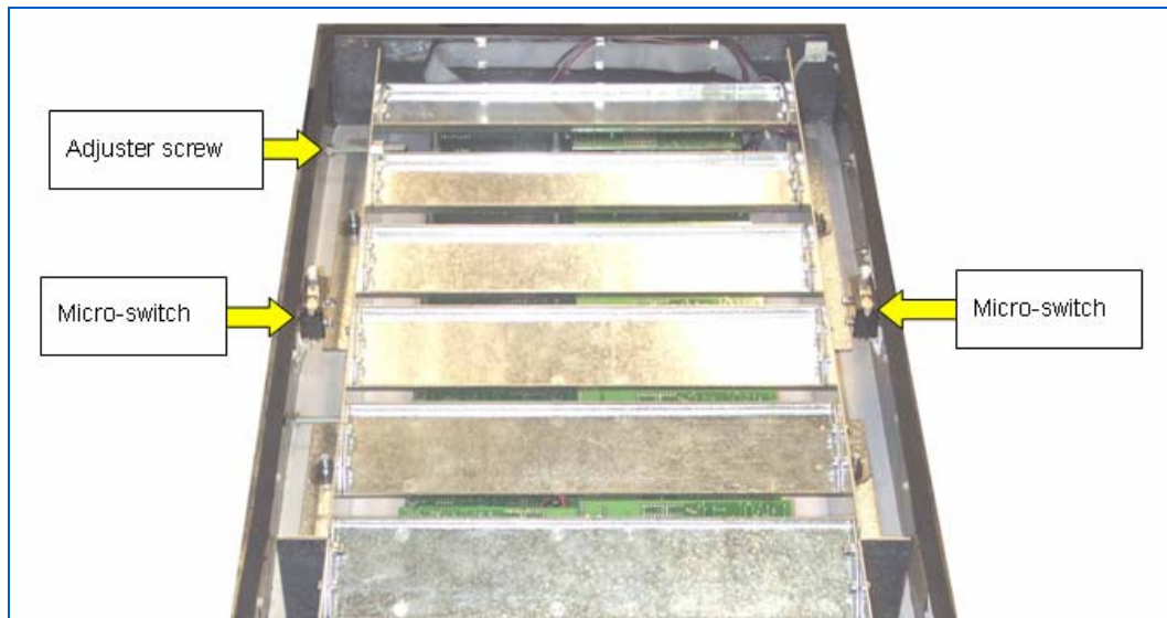
Figure 295: Diode Array Box
