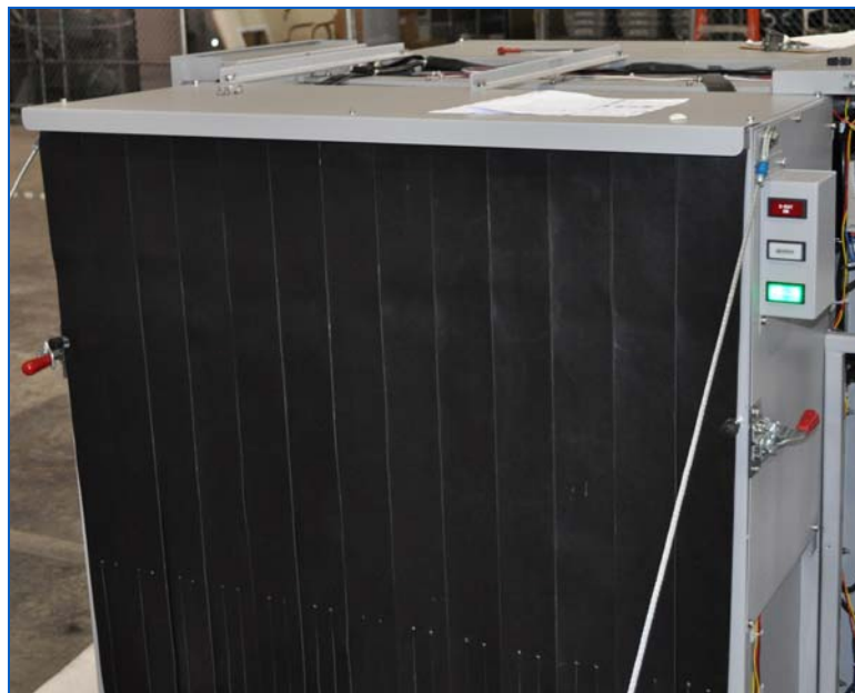
Figure 23: Curtains and Light Indicator Box
