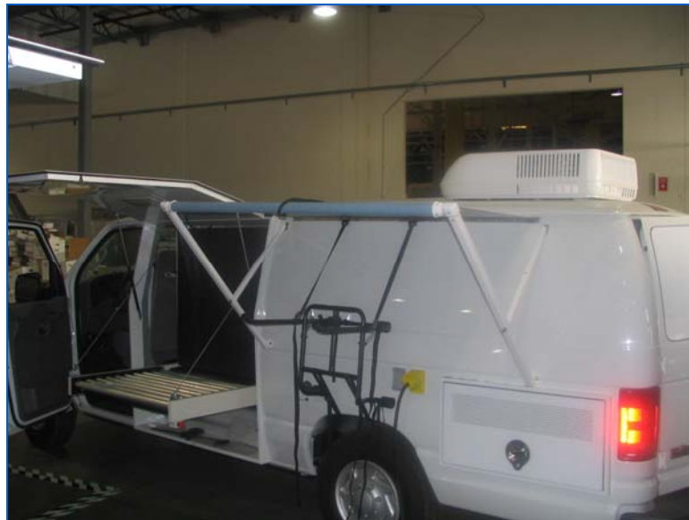
Figure 66: Conveyor Door Open
