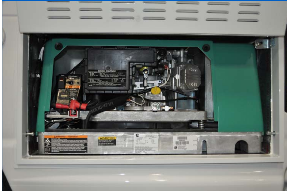
Figure 71: Auxiliary Power Generator Set (Genset)
