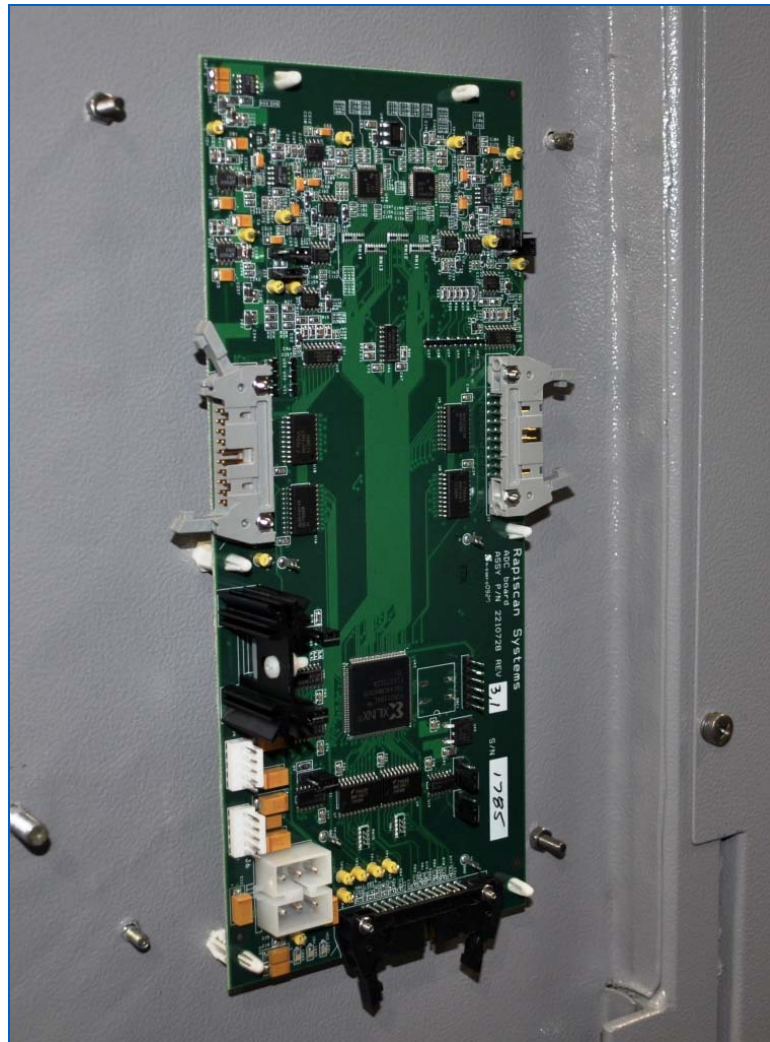
Figure 314: Analog to Digital Conversion board (ADC)
