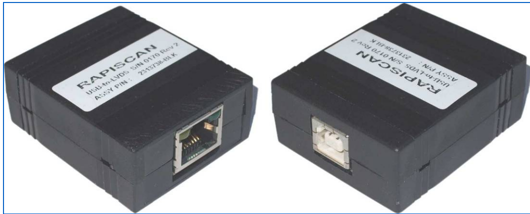
Figure 243: LVDS to USB Converter
