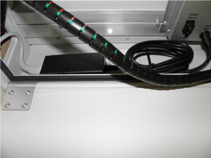
Should it be necessary to put the power supply inside the cross piece do as follows:
