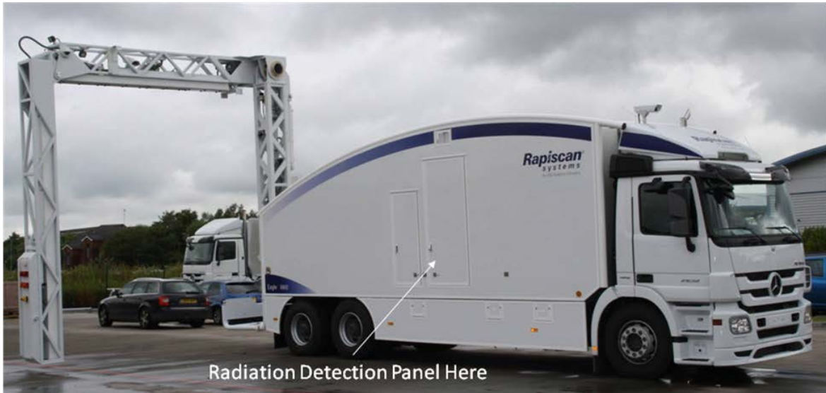
Figure 2. Eagle M60 with Boom Deployed for Scanning
