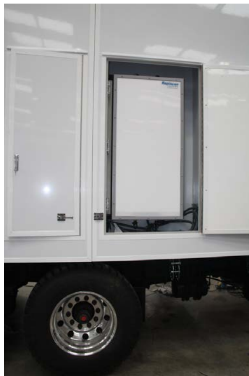
Figure 3. Radiation Detection Panel Installed on Side of Eagle M60
