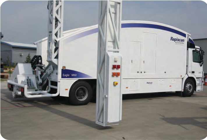
Rapiscan's Rad-Nuke detectors are designed for the integration into Mobile platforms, such as the Eagle M60
