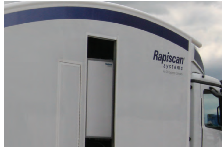
Rapiscan's Rad-Nuke detector visible within the Eagle M60
