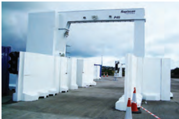
Eagle® P45 with radiation shielding.
