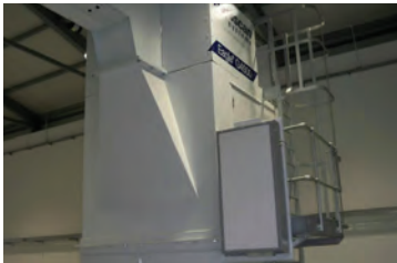
Eagle® G60 with integrated radiation detection panel.
