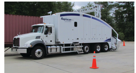
Rapiscan Eagle® M60 scanning with Auto-Z™ enabled.
