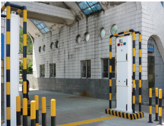
Rapiscan's TSA VM250 detects radioactive emissions on moving vehicles
