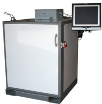
TSA BM285 waste monitor with door closed
