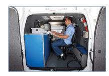
The Rapiscan MobileCheck™ 636SV is a state of the art self-contained mobile X-ray screening unit with a large tunnel opening. With an innovative design the ability to rapidly deploy baggage and parcel inspection at any location with one complete unit is possible. The Rapiscan MobileCheck 636SV can be deployed and operated in three different modes, from either side of the van or in a pass through mode.
