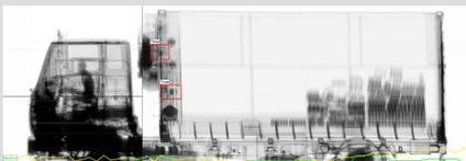
The Eagle T60 high-energy X-ray image with optional CabScan mode and integrated radiation detection
